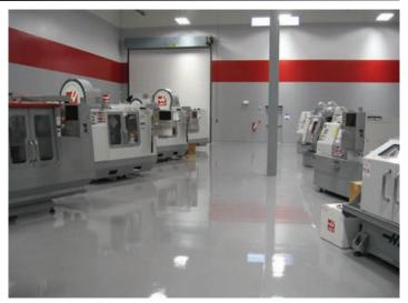
Stonhard installed a seamless, epoxy floor system in the Haas CNC shop. This extremely durable floor is also chemical, abrasion and slip resistant.
